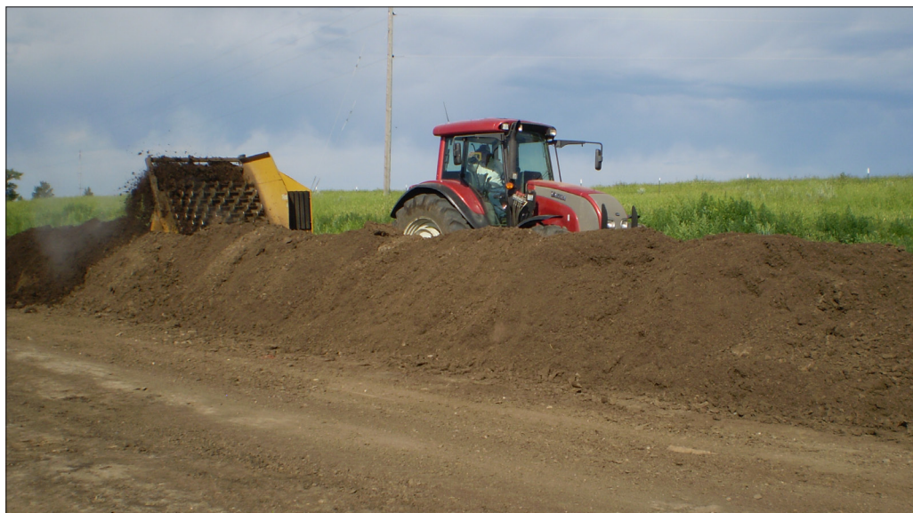
FIGURE 5. Tractor with compost turner near Havre.
