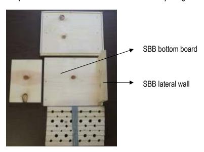
Step 2 - Determine the location of the second lateral wall by placing the SBB nesting block in its position.
