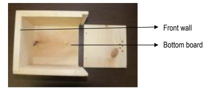
**Step 4** - Secure the lateral walls to the front wall by using six 11/4" screws.
