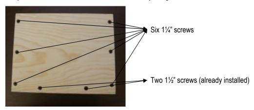
**Step 5** - Secure the back wall to the bottom board by using two  $1\frac{1}{2}$ " screws.
