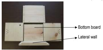
**Step 2** - Secure the second lateral wall to the bottom board by using two 1½" screws.
