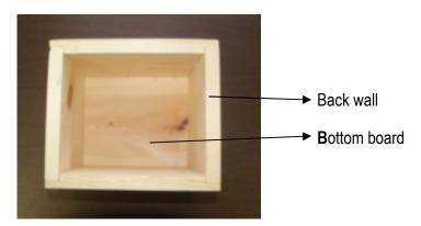
**Step 6** - Secure the lateral walls to the front wall by using six 11/4" screws.
