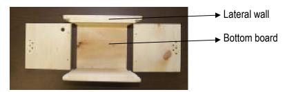
**Step 3** - Secure the front wall to the bottom board by using two  $1\frac{1}{2}$ " screws.
