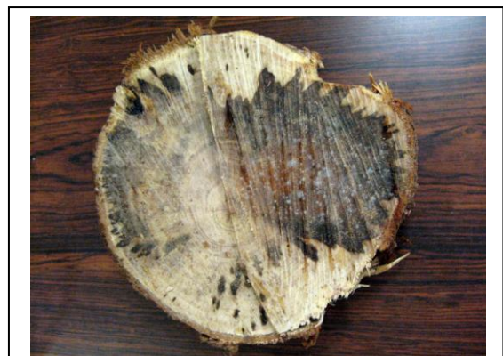
11-24. Superficial fungal growth not originally present.
