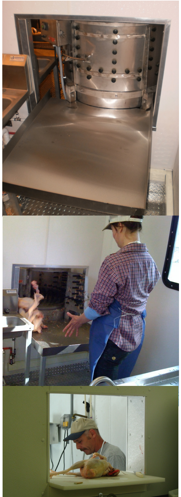
Top: Pass-through on enclosed Massachusetts MPPU, with kickout door from plucker Middle: Kickout door in action (a plastic “backstop” was later added to the catch table) Bottom: Pass-through window, Stone Barns Center
