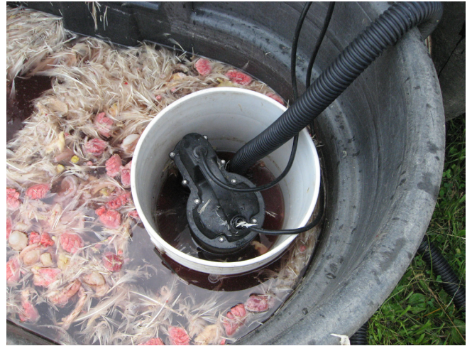
“Offal soup,” the product of mingling solid processing wastes with wastewater. Here a sump pump is sending the liquid waste to a compost pile, with a screen preventing (or attempting to prevent) the solid waste from clogging the pump.
