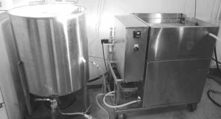
This computer-controlled apple cider pasteurizer is another of Lou's inventions developed through a SARE research grant. Photo by Merby Lego
