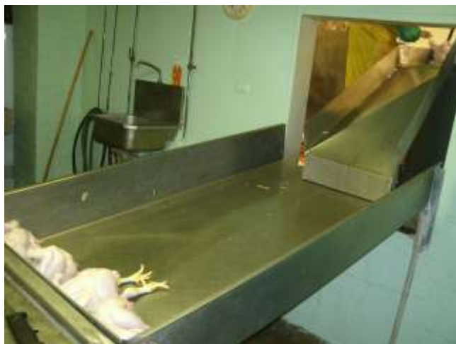
Chickens are sent down the chute from the picker in the “dirty” area on to a table where they can be rinsed and feet clipped before being moved to the evisceration table
