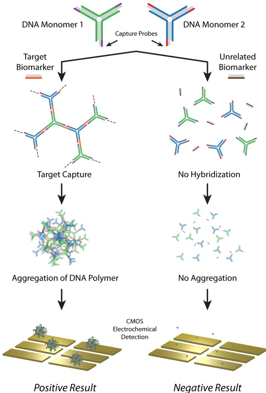
**Figure 1: Overall scheme as proposed in 2011.** DNA nanostructures are prepared with capture probes, which can recognize and bind to pathogen target biomarkers.
