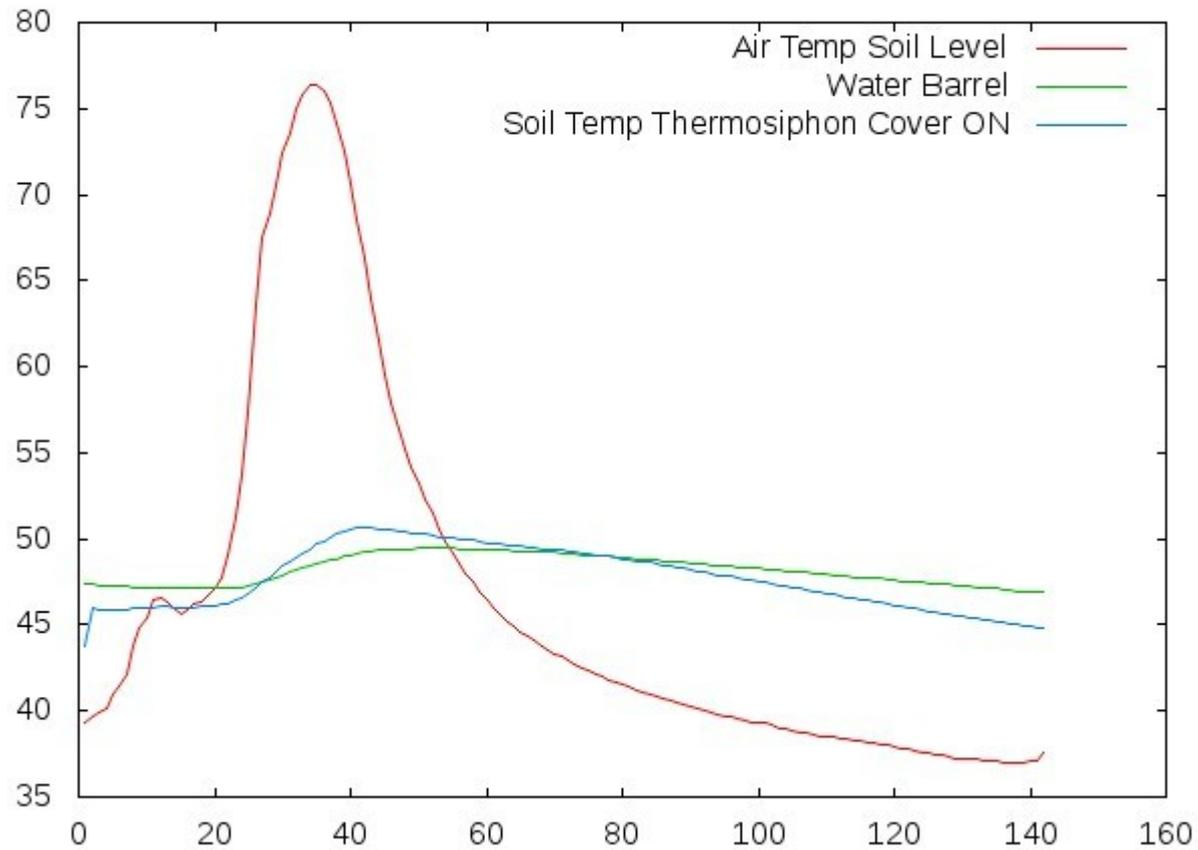
Without solar heating of thermosiphon water, soil temp remains close to water barrel temperature.
