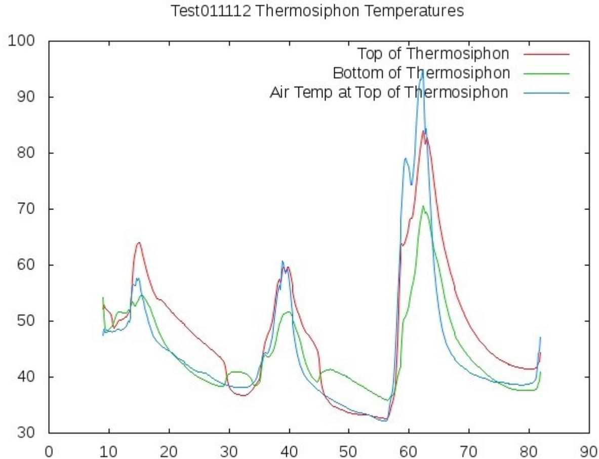
First two days cloudy, last sunny. First day, top temp exceeds air temp; first two days, bottom temp exceeds top late in day; last day, top temp remains above bottom, almost 15 deg difference.
