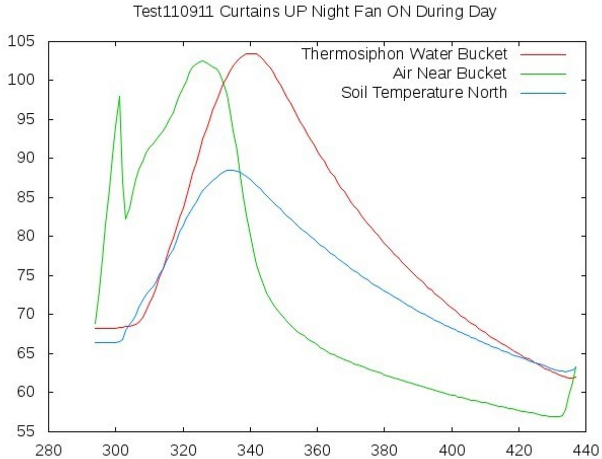
Notice Thermosiphon water bucket temp similar to air temp, with time lag.
