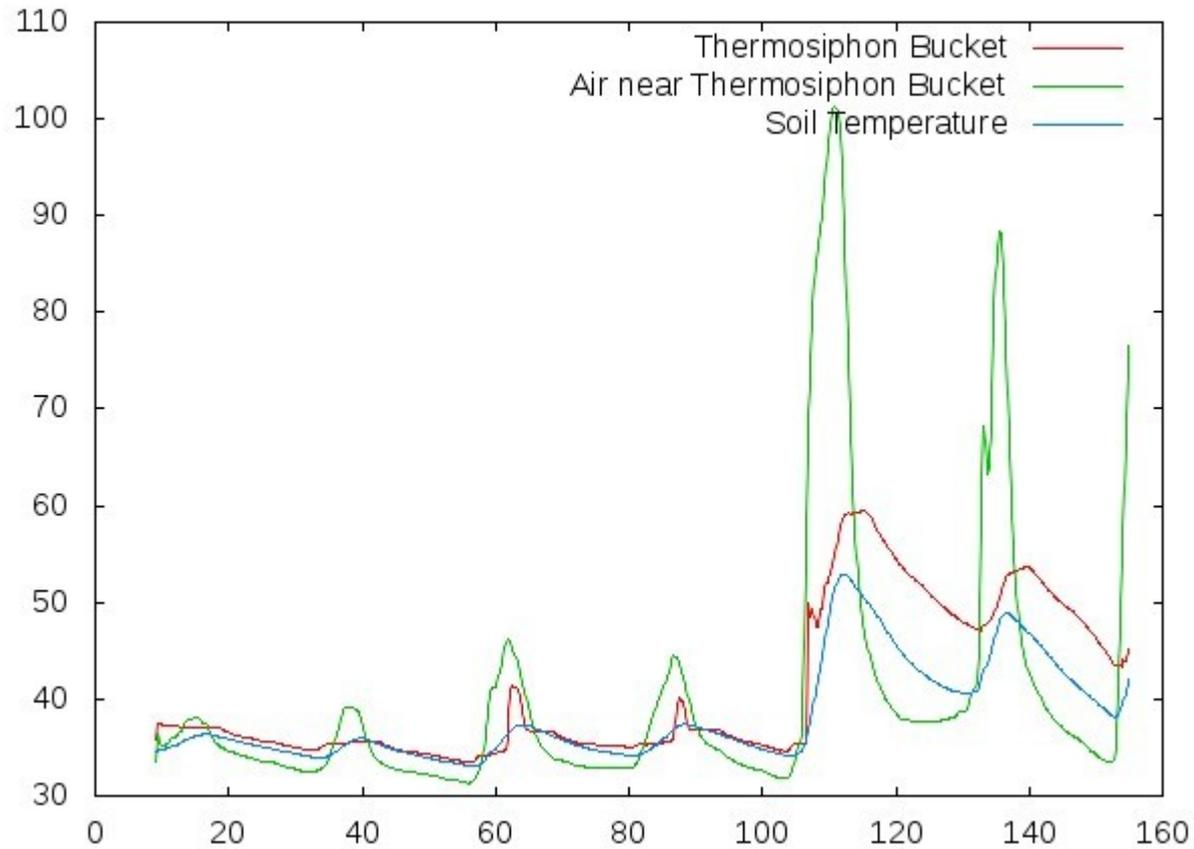
Thermosiphon Bucket Temperatures less than air temperatures near Bucket, much less for sunny days, when Solar Collector Covered.
