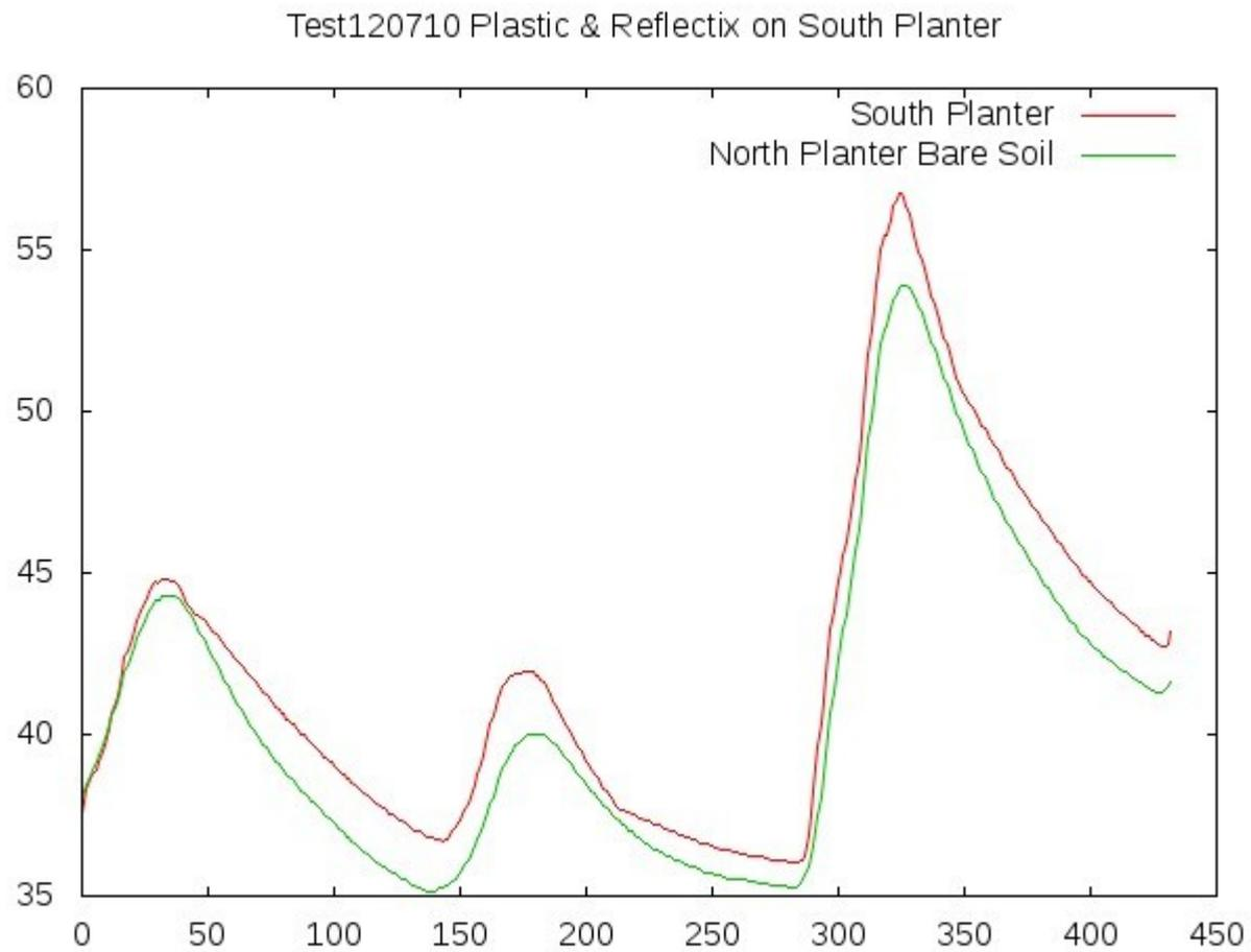
Kinks in south planter soil temp due to covering with Reflectix
