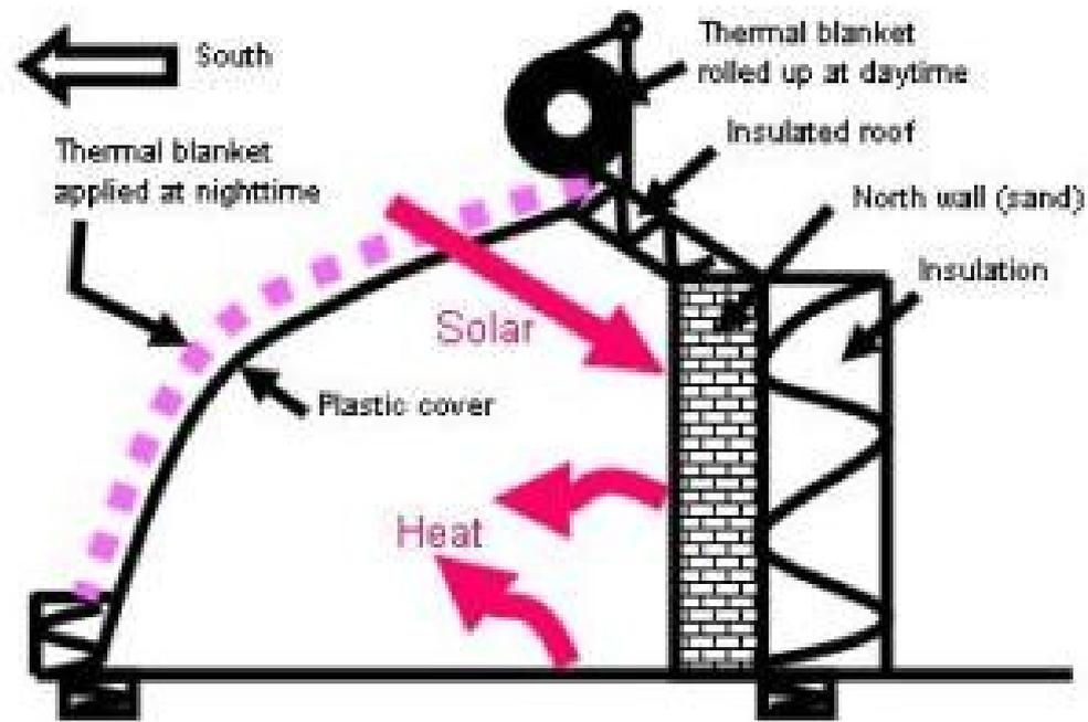
Figure 1. Schematic illustration of a solar energy greenhouse
