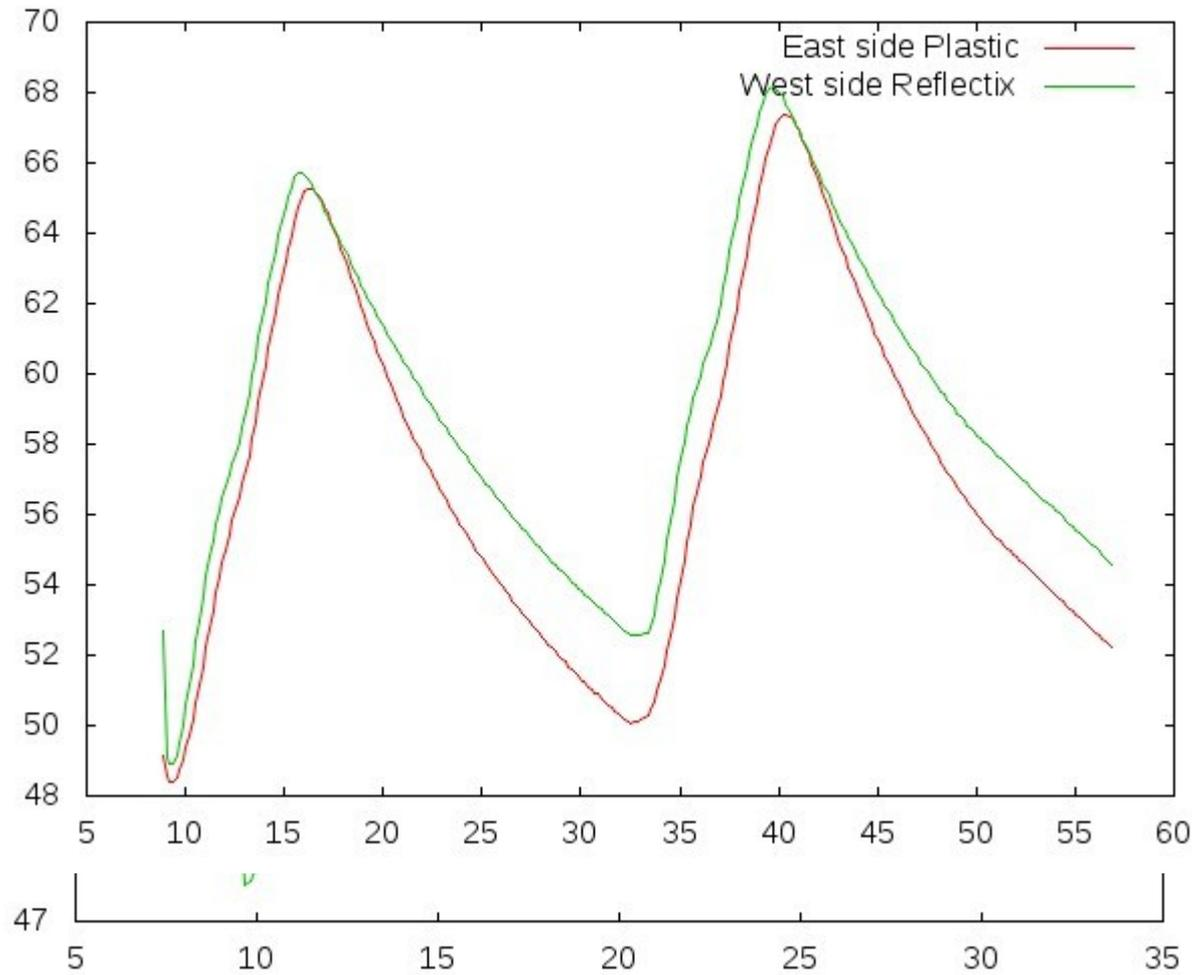
Even when low over soil, Reflectix provides a 3 degree boost with smaller conduction and radiation losses
