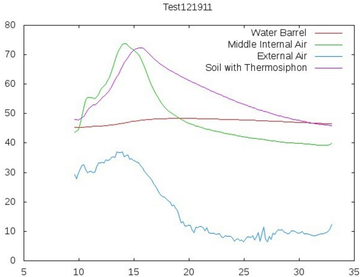
Soil Temp with Thermosiphon over 20 degrees higher than water barrel temp, which changes little.
