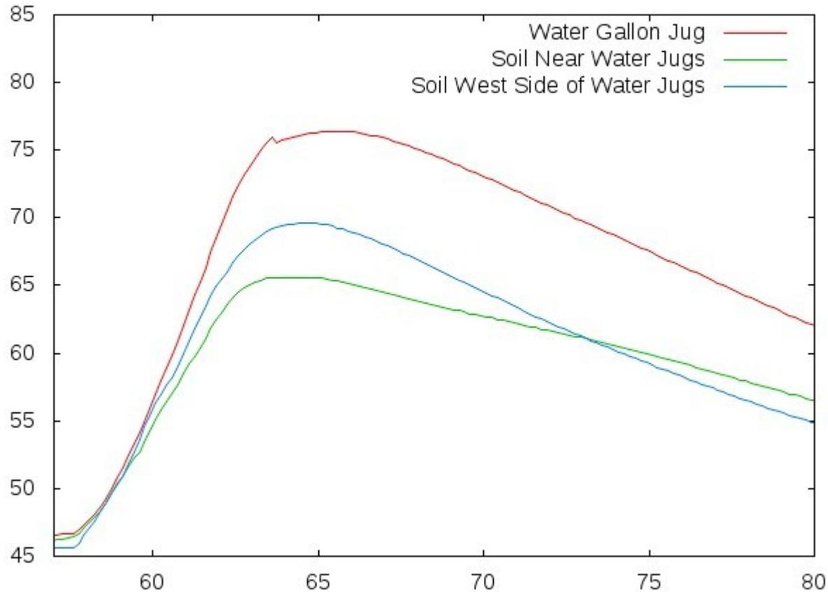
Soil near 4 1-gallon jugs covered by Reflectix at night exhibits 9 deg F drop over night; Soil covered by Reflectix shows 15 deg F drop over night.
