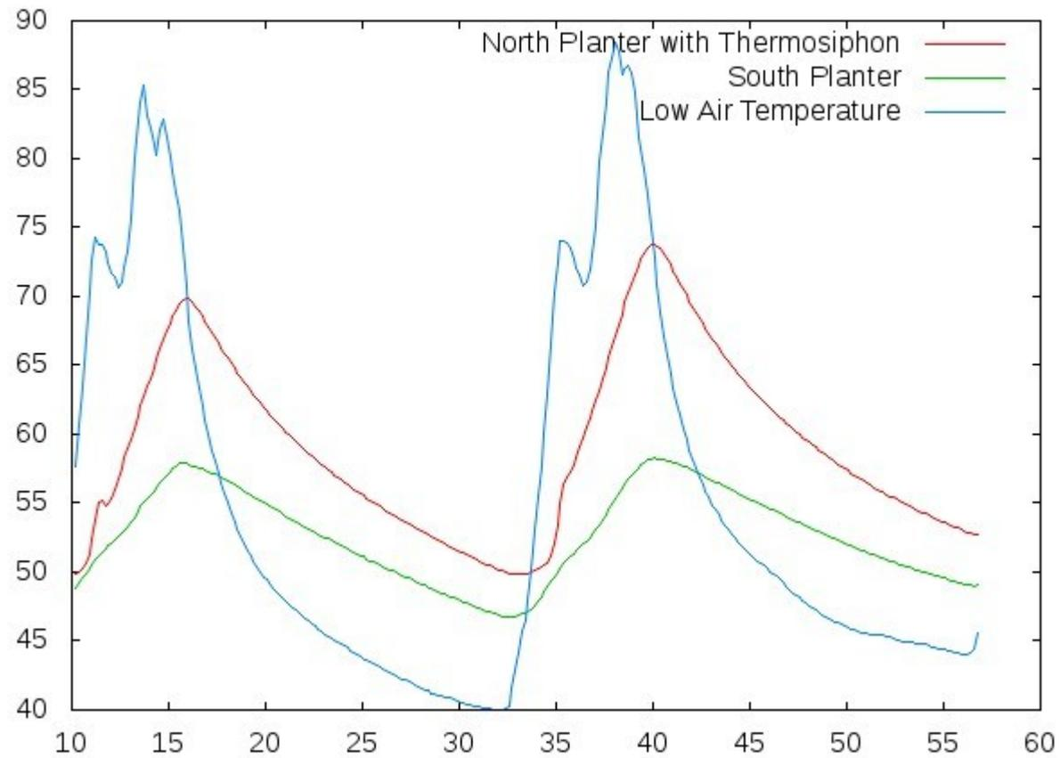
Thermosiphon working – 15 deg peak difference, 4 deg minimum
