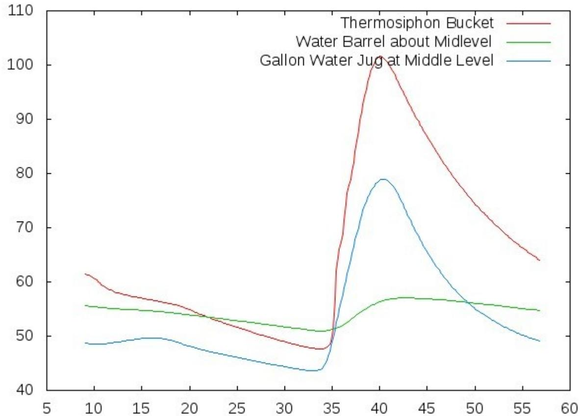
Gallon Water Jug gains and loses much more heat energy than 55-gal Barrels. Surface to Volume ratio 5 times greater for Gallon Water Jug, which is about the increase in heat exchange per unit volume.
