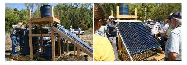
Some of the workshop attendees during the demonstration of anaerobic digester and evacuated tube solar heating system
