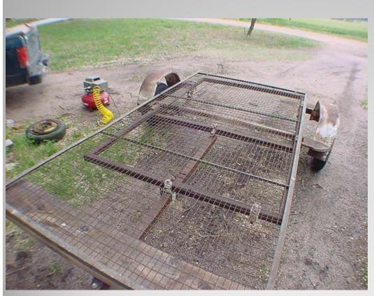
Base is welded mesh farm panel, secured on old boat trailer.
