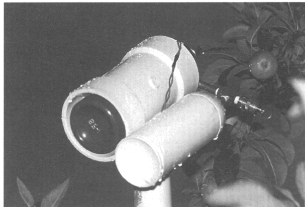
This microsprayer releases pheromones in puffs of atomized liquid from pressurized canisters. Photo: J. Ogradnick.
