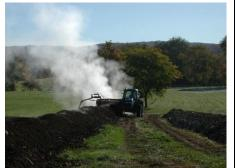
When loads containing food scraps are received, they are immediately mixed with ground brush, chips, and leaves in small batches at the far end of the compost pad area. These mixed materials are formed into 140-foot long windrows (elongated piles), along with additional leaves. Some renderings are also accepted and composted separately, strictly for use on farm fields.
