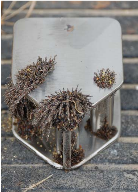
Figure 1: Ferrous metal debris collected by the magnet in the nozzle.
