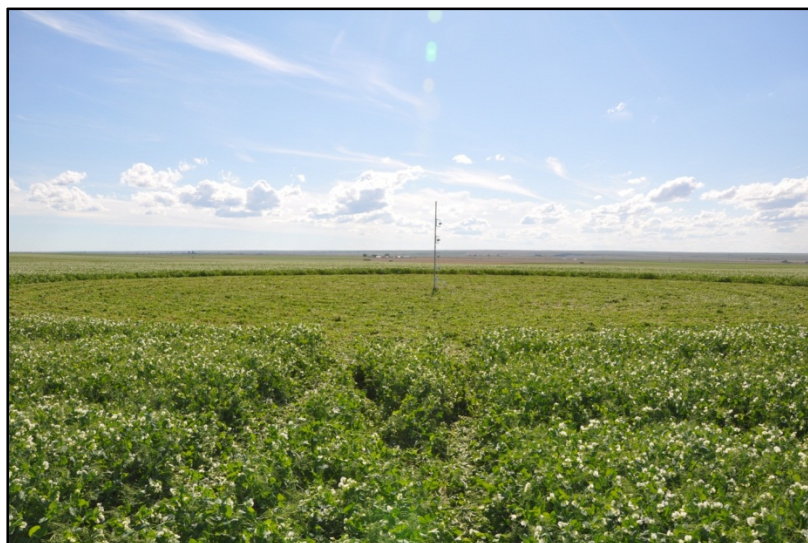
Figure 7. Field peas were terminated at the early-pod stage in 2011 (top) and flowering in 2012 (bottom) at field sites near Havre, Montana. A mast with Leuning samplers was erected inside of the circular plots to trap \text{NH}_3 loss according to the integrated horizontal flux method.
