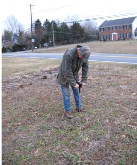
Figure 13 Russell Reeder using a soil penetrometer to measure compaction.
