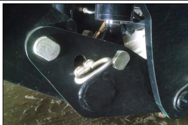
Figure 01 (above): This pin position lets the arms move up and down slightly in response to changes in the terrain. It also allows one arm to move up or down while the other stays in place, which helps on sloped terrain. Inserting the pin in the other opening firmly locks the arms in place.
