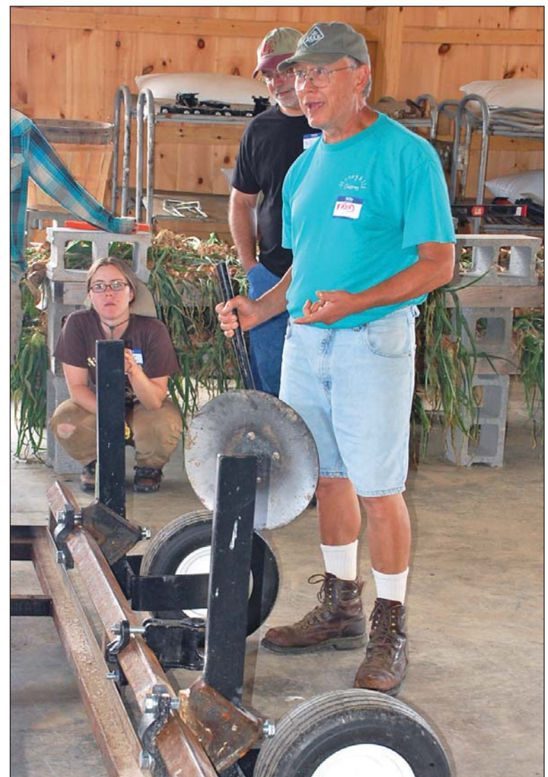
Attaching hilling discs (as held in Fred Forsburg's hand) or other equipment is possible with the new platform design.
