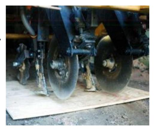
The front disk slices the residue, the shank (whose depth is adjustable) loosens the soil without inverting or incorporating the residues, the tube delivers organic fertilizer, and the fluted coulter mixes it into the planting slot. A no-till transplanter with specially-designed press wheels then places seedlings or seed potatoes into the slot.
