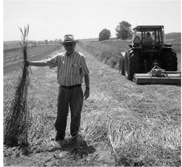
Figure 2. The roller-crimper (left) has been developed specifically for no-till management of high biomass cover crops. The flail mower (right) is a versatile tool, in that it can be used to generate even, finely chopped mulch, or can be operated with the PTO off to function as a roller, as shown here.
