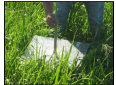
Homemade falling plate meter. (Practical Farmers of Iowa)
