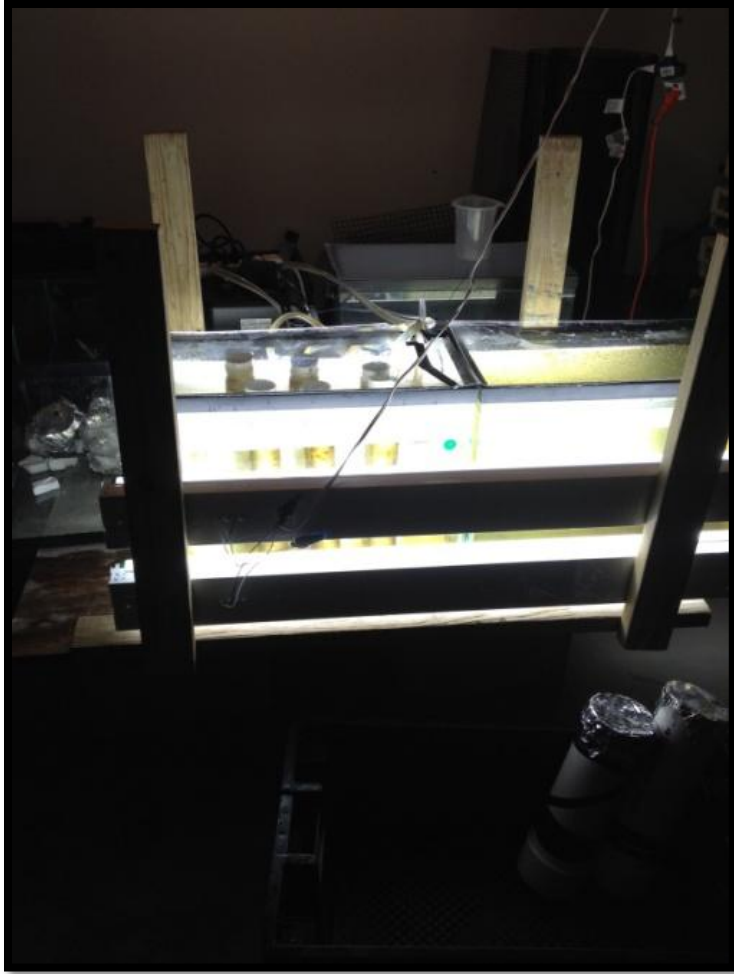
Figure 6. Nursery setup showing kelp seed string within the aquaria, and supplemental lighting lateral to each tank.
