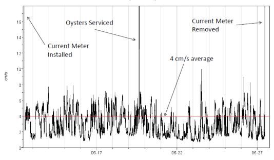
Figure 12. Current at the growout site. Average is 4 cm/s, with short pulses to 8-10 cm/s.
