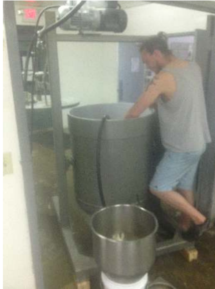
Illustration 6: Skimming nut meat off top of Barrel Float
