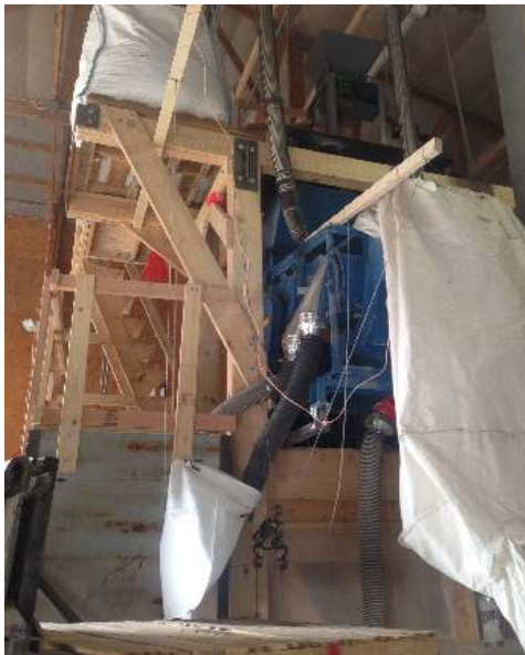
Illustration 5: Seed Cleaner and Cracker set up
