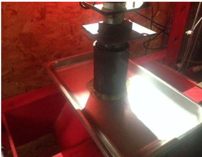
Illustration 7: Oil Pressing tests for black walnut and hickory nut
