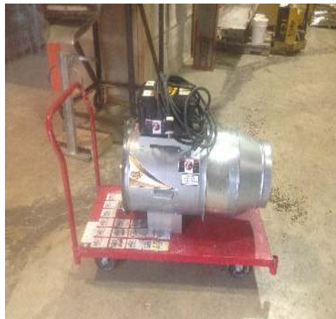
Illustration 2: Dryer with reducer to attach to totes
