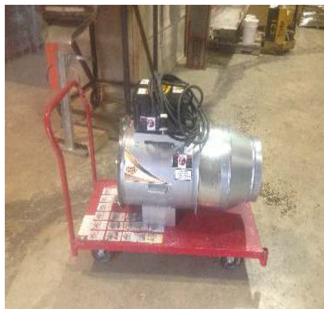
Illustration 2: Dryer with reducer to attach to totes
