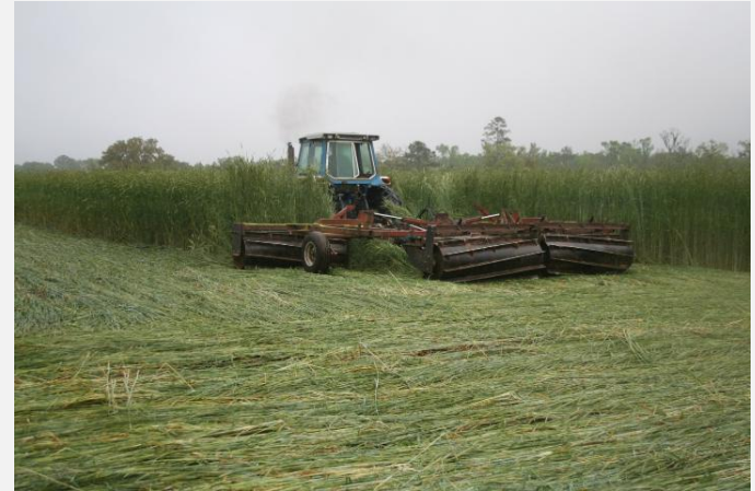
Cereal rye cover crop rolling/crimping in late March 2011 at Brock Farm in Monticello, Florida. Custom roller/crimper design and fabrication by Kirk Brock
