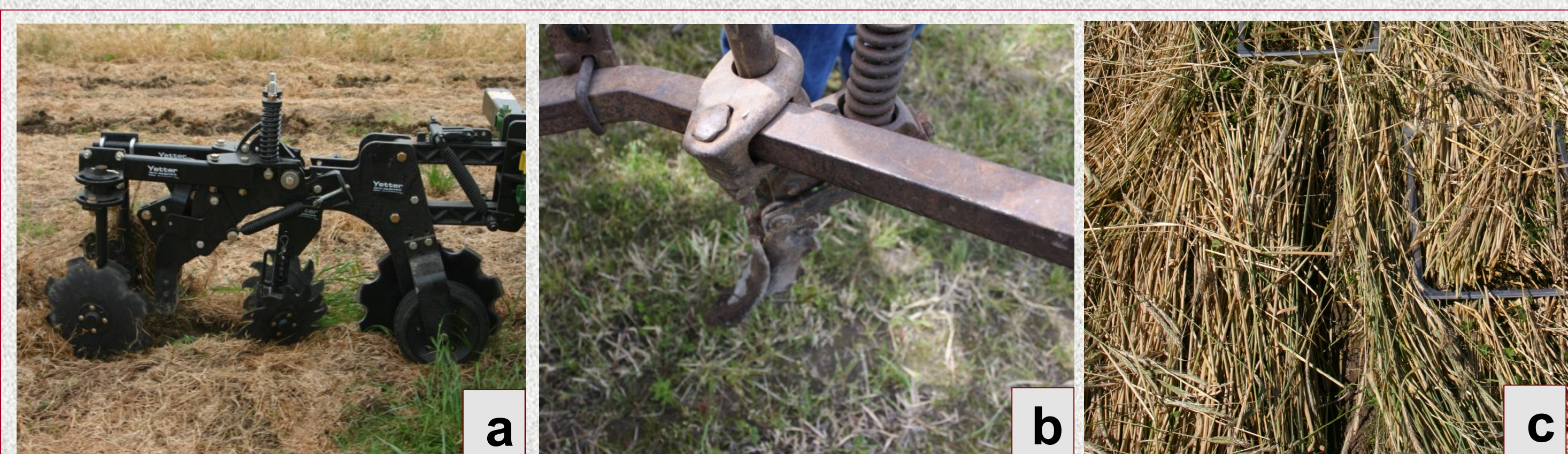
Figure 2. Reduced tillage plots were prepared for transplanting with a Yetter Strip Tiller (a) or with a custom “planting aid” tool (b) that leaves a 5 cm wide by 10 cm deep swath (c).
