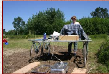
Figure 3. CO 2 was measured with an infrared gas analyzer on In-row and Out of row chambers.
