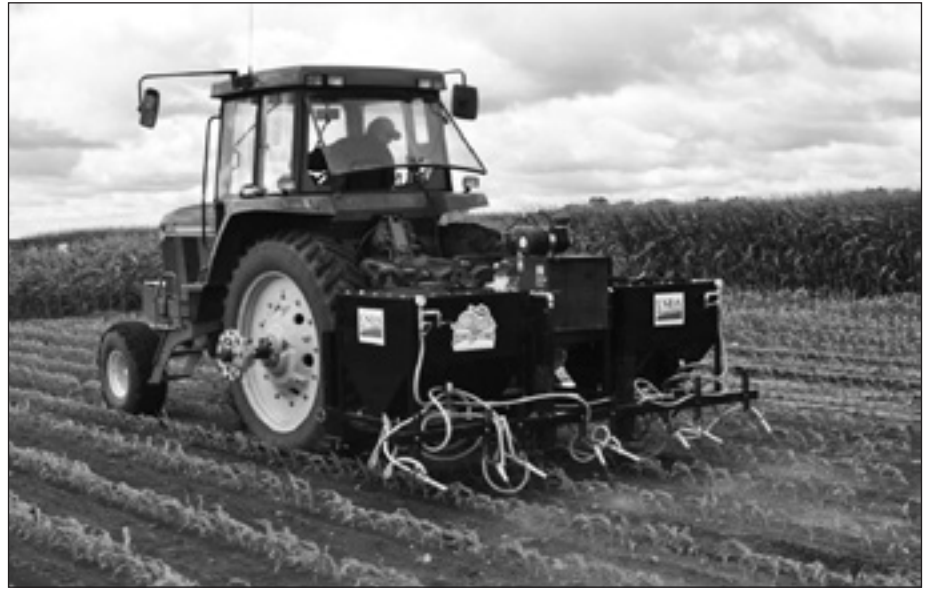
The four-row, eight-nozzle PAGMan provides selective, post-emergence, in-row weed control for corn, soybean, and other crops grown in widely spaced rows.
