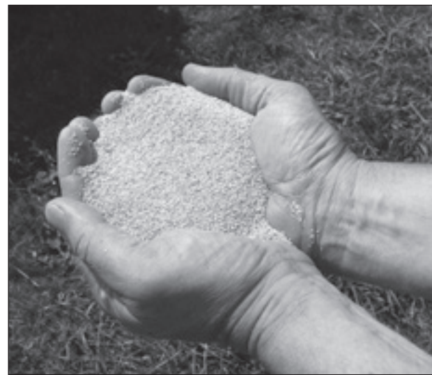
Ground corn cobs make an effective grit for "sandblasting" weeds. Any gritty material that is about 0.5mm works with the PAGMan system.
