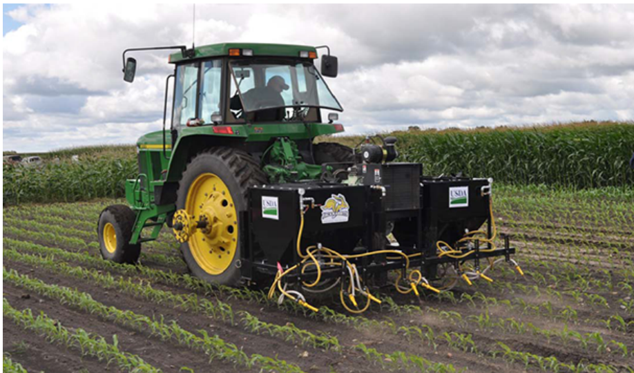
The four-row grit applicator in action, driven by Charles Hennen. (Photo: Frank Forcella)
