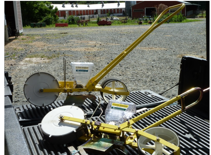
Clean Seeder gear settings: R9, F14 Roller: X12
