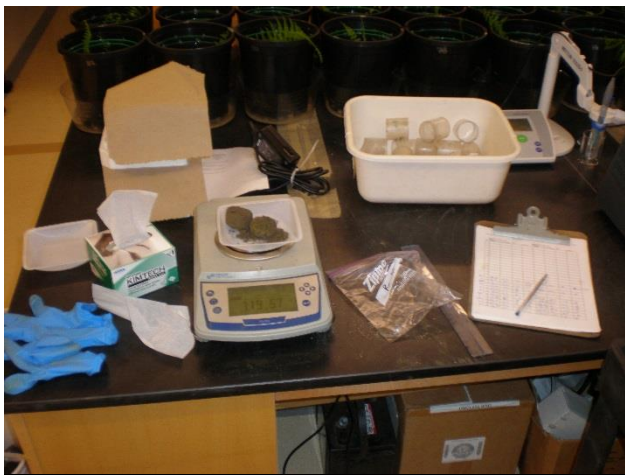
Figure 52. Measuring Bulk Density in Lab
