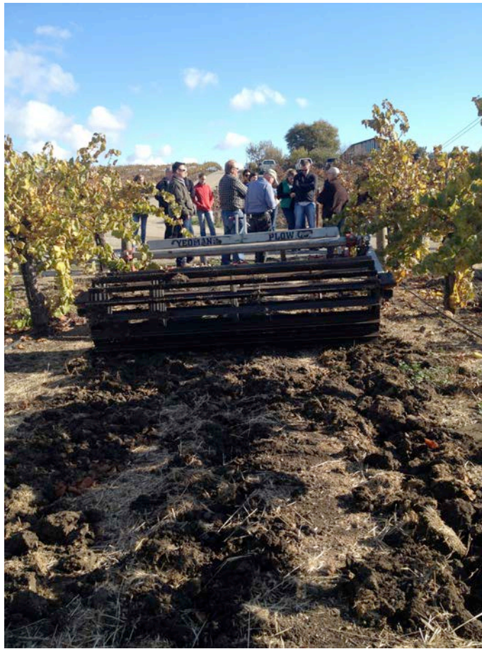
Yeoman's or keyline plough used at Wolff Vineyards to enhance soil health and water penetration
