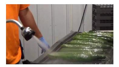
It was important that we used a sprayer head and sufficient water pressure that the produce was washed but not bruised. Since they are greenhouse grown we didn't have as much soil as field grown, but we tested the system on some field grown produce and it successfully washed off visible soil.
