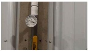
We used regular garden hose and sprayers and installed a thermometer in the line so we could determine the water temperature.
