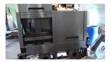
Above and below- the side of the unit, we will have to replumb it to spray wash, sanitizer and rinse (if necessary) water.
