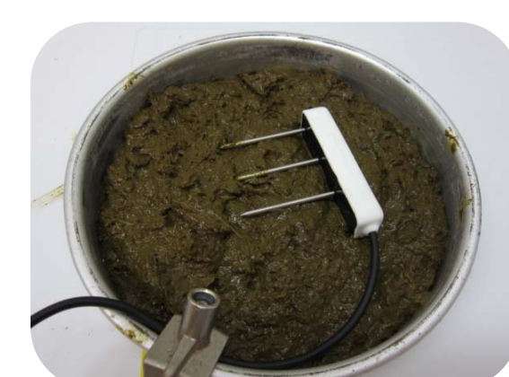
GS3 moisture sensor installed at the center of the calibration ring
