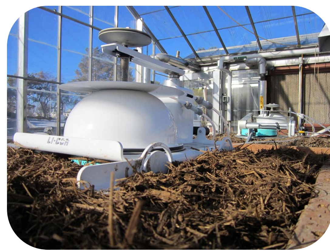
Closed dynamic chambers (CDC) coupled with a multiplexed Fourier Transformed Infrared (FTIR) spectroscopy gas analyzer provided gas flux estimates.
