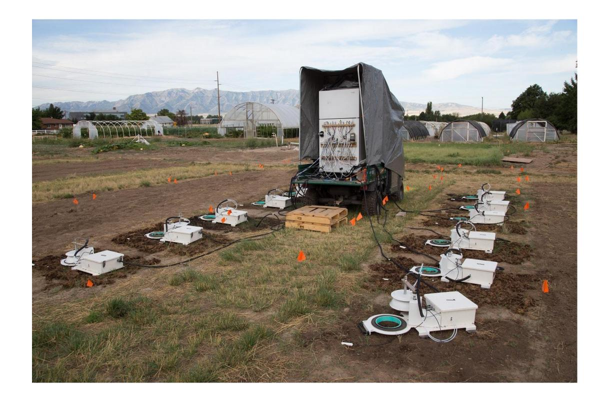
In addition to gas emissions, primary meteorological factors affecting evaporation, including temperature, atmospheric pressure, relative humidity, and solar radiation were monitored (below).
