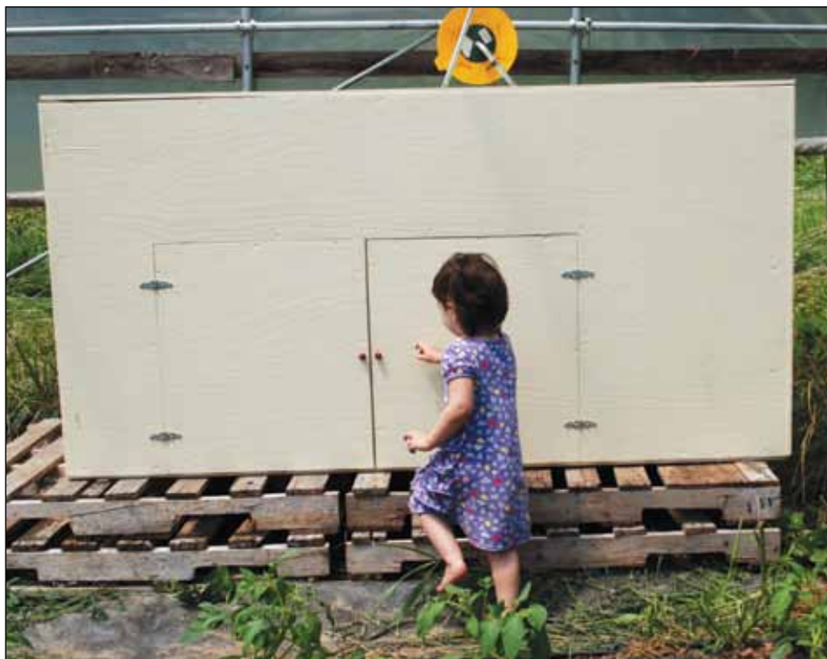
The electric dryer houses 18 trays in two stacked columns.
