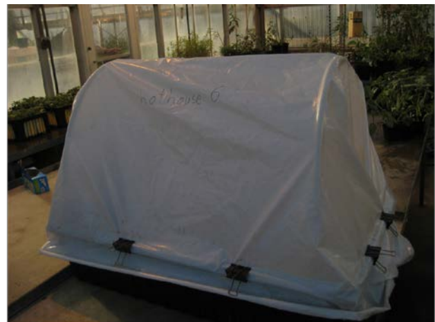
Fig. 4. A finished humidity tent with the plastic sealed at the sides and ends with 2 inch paper clamps.
