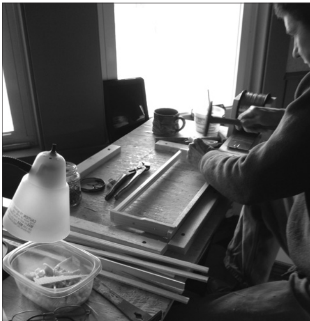
Cindy assembles a wedge-top/divided-bottom frame.
