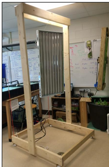
Figure 3. Mobile light tower with rolling frame (left) and wall-mount light tower (right) for vertical tower system.
