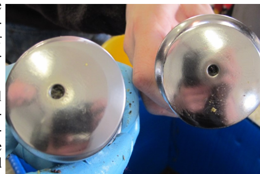
Figure 9. Scuffed screws (left) need to be polished (right) to increase press efficacy.
