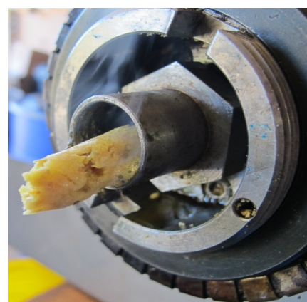
Figure 12. Close-up of collar head and nozzle with too-hot soy meal.
