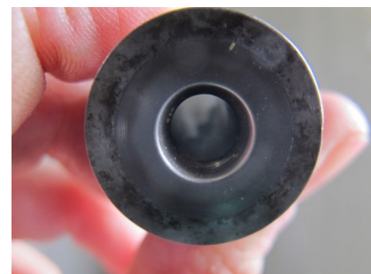
Figure 5. The AgOil M70 comes with three different sized nozzles: 220, 250, and 280.
