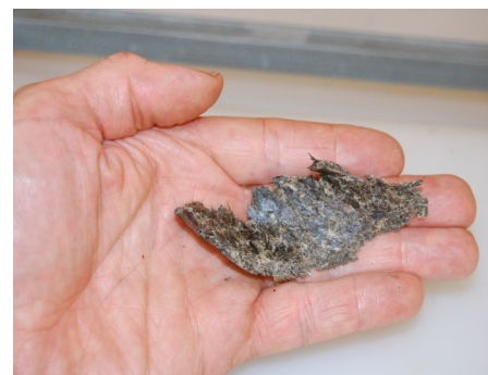
Figure 7. This was the only press evaluated in this study that produces meal in the form of flakes, rather than pellets.
