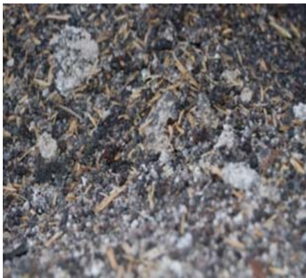
Fig. 5: Mold in canola resulting from condensate formed as temperature lowered
