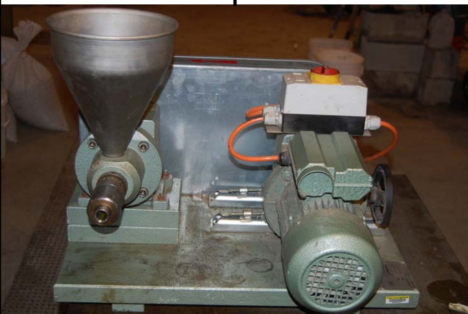
Figure 1.1.2: Small expeller press for extracting oil from seed.
