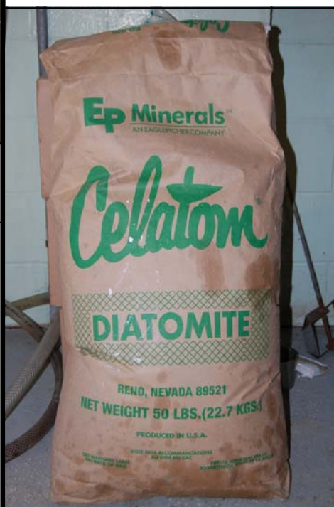
Figure 2.4.12: 50 pound bag of diatomaceous earth (DE). For this vendor designation FW-14 works well for filtering vegetable oil.
