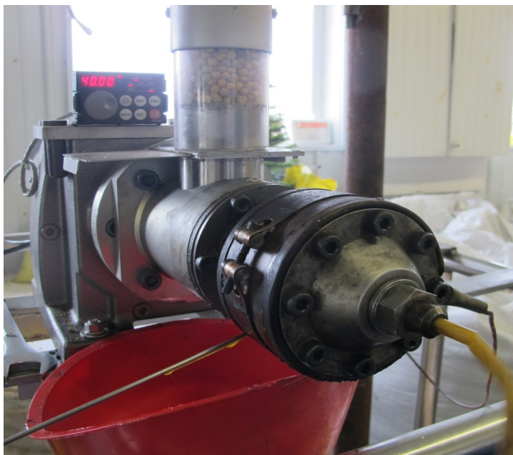
Figure 4. AgOil 70 press at 40 RPM, pressing soybeans.
