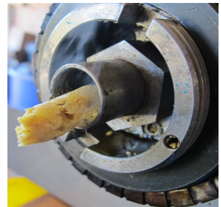
Figure 12. Close-up of collar head and nozzle with too-hot soy meal.
