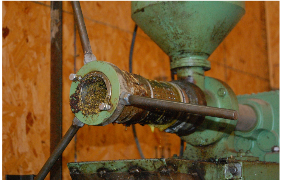
Figure 6. The Keller press has a single barrel and drive.
