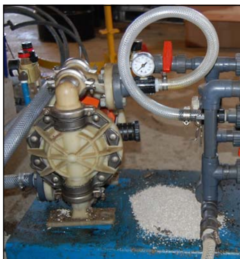
Figure 2.4.10: Air operated diaphragm pump on filter press.
