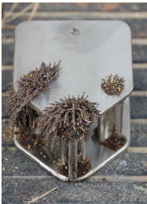
Figure 1.1.1: Ferrous metal debris collected by the magnet located before the press.
