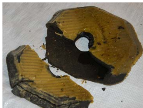
Fig. 9: Block of foots collected from between two filter press plates. The yellowish colored material is filtering media coating (diatomaceous earth) initially placed on filter plate cloth while the dark colored materials are the foots.
