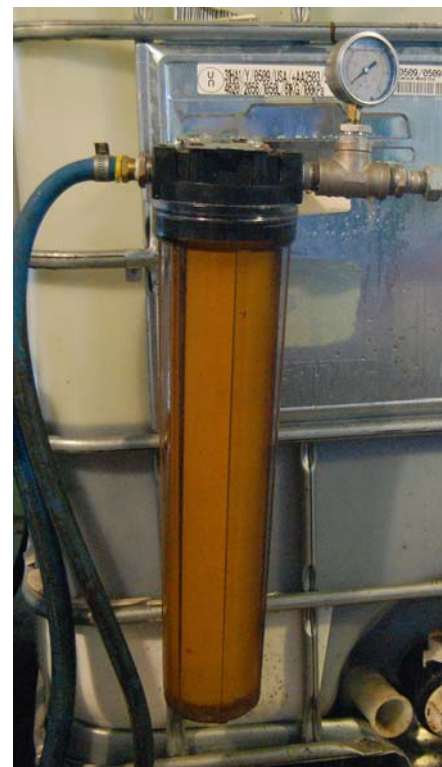
Fig. 7: Cartridge filter with clear housing used as final filter for fueling with straight vegetable oil
