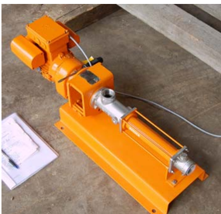
Fig. 11: Electric screw pump for filter press
