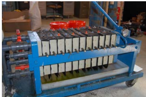
Fig. 8: Filter press; a series of filtering plates are pressed together by manual screw or hydraulic pressure.
