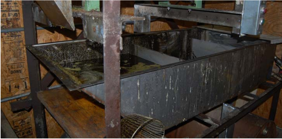
Fig. 3: In this tank pressed oil flows slowly from left to right. The oil passes across two partitions, allowing particles time to settle. Most of the settling occurs within the first partition.
