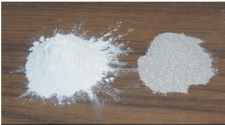
Figure 4: Two different types of bleaching clay. Shown on the left is a sample that is mixed with the oil, heated, and put through a filter press. On the right is a sample that is used as a filter in itself, which the oil is passed through. In both cases, the unwanted components in the oil are bonded with the clay, removing them.
