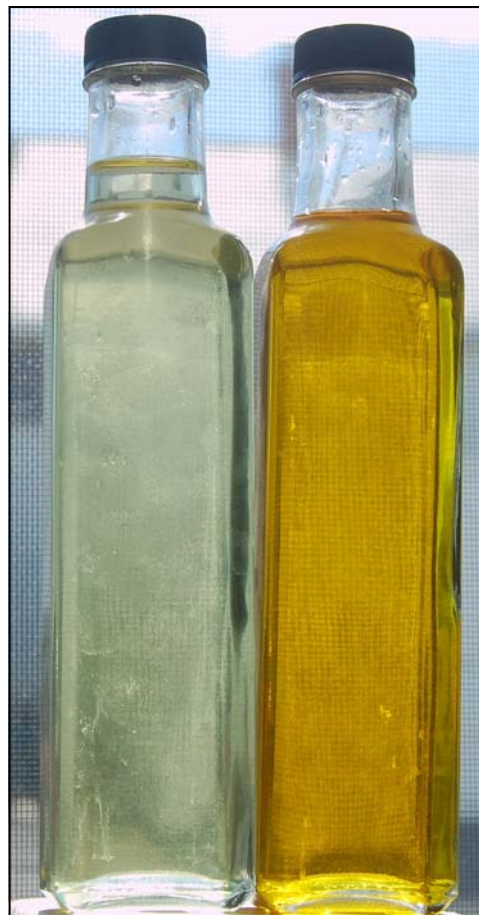
Figure 5: Bleached canola oil (left) and un-bleached canola oil (right) are very different in color due to the natural colorants removed during bleaching.
