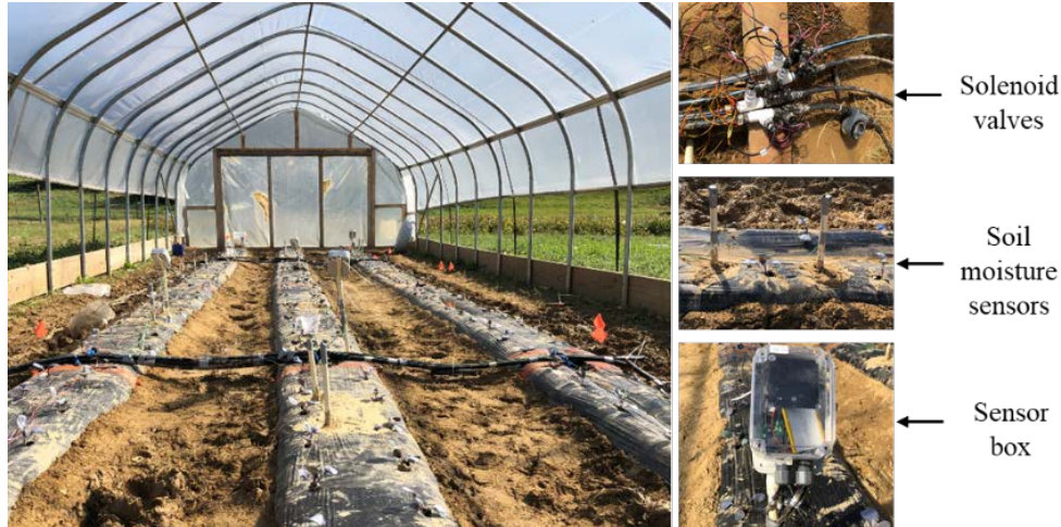
Figure 1. An IoT-based irrigation setup in a high tunnel vegetable crop system
