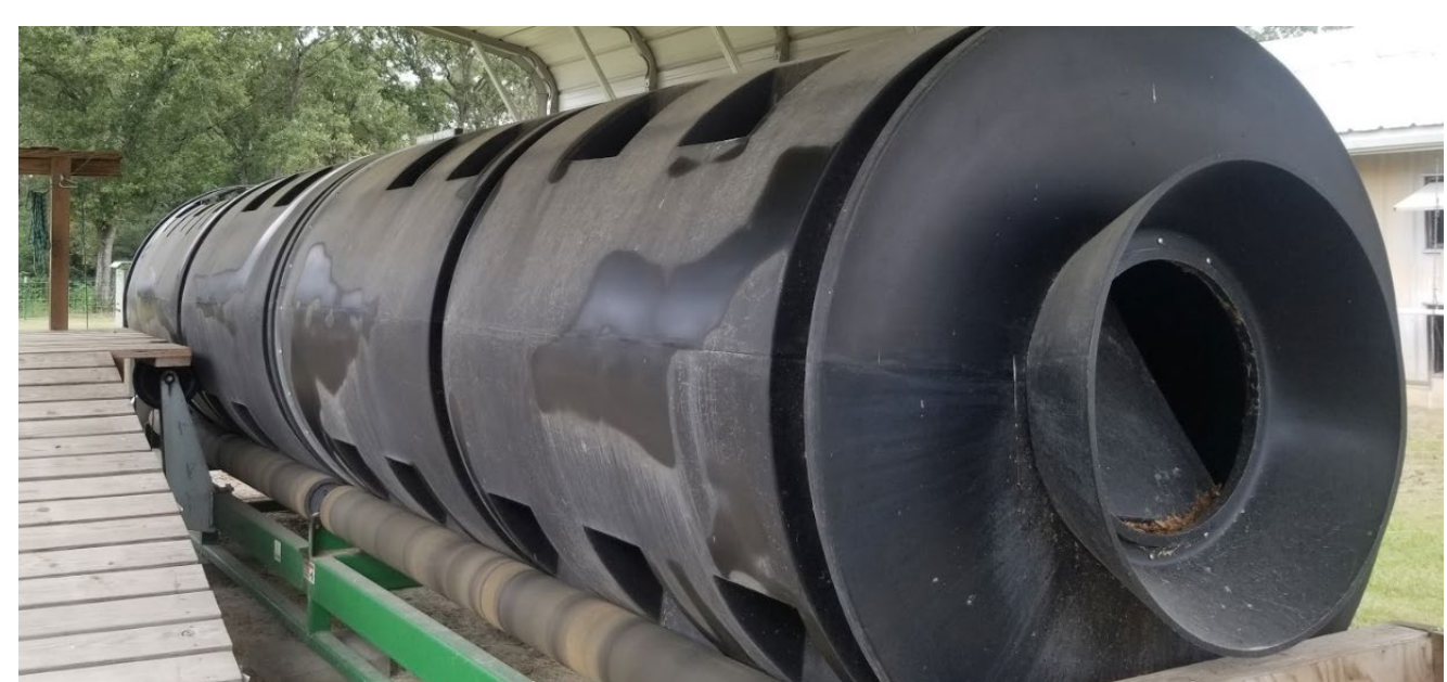
Fig. 2: Barrels of SCG from a cold brew coffee manufacturer were loaded into the EcoDrum® daily, for three consecutive days.
