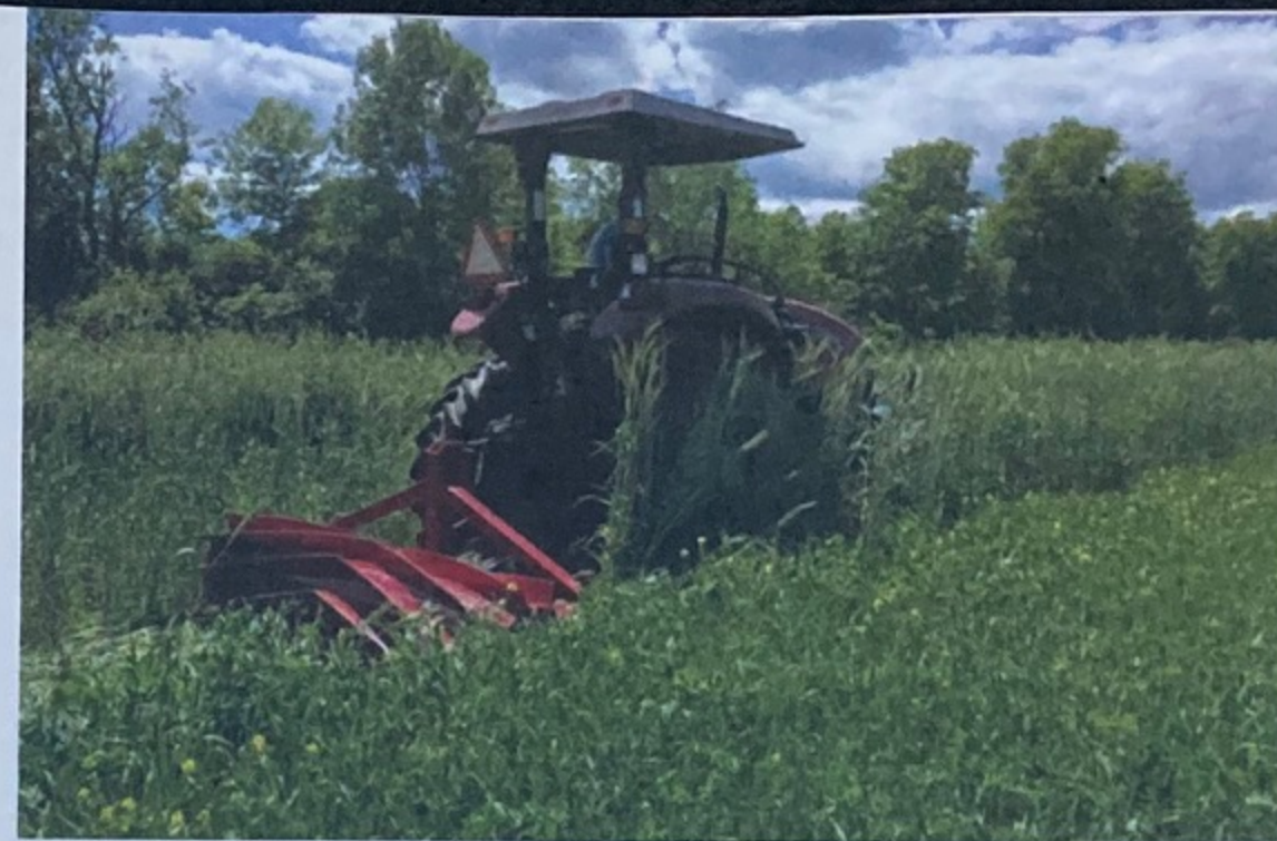
The roller-crimper is a valuable tool for organic vegetable production.
