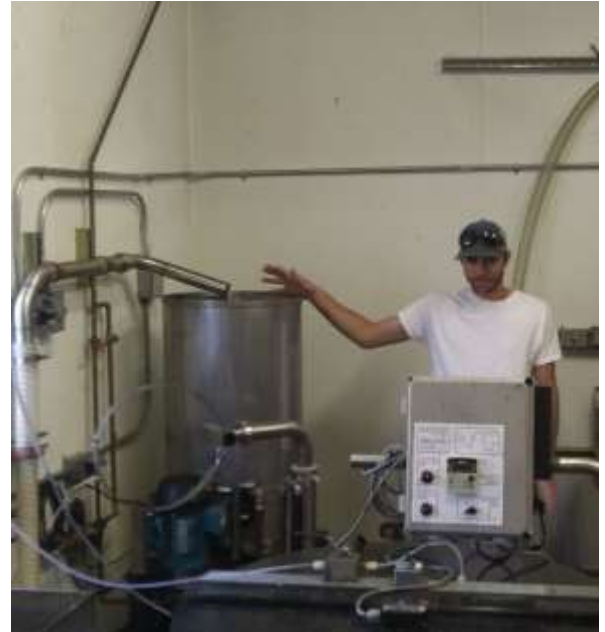
Garrett Wentzel demonstrates preparing a frame from a hive “super” for honey extraction. The wax cap is removed with a knife before being inserted into a centrifuge (left). As the centrifuge spins, honey and wax are thrown to the inside walls of the centrifuge and pumped to a heated separator (right) where wax and impurities are filtered from the honey.
