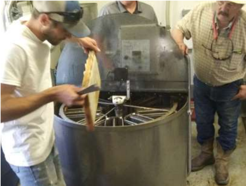
Garrett Wentzel demonstrates preparing a frame from a hive “super” for honey extraction. The wax cap is removed with a knife before being inserted into a centrifuge (left). As the centrifuge spins, honey and wax are thrown to the inside walls of the centrifuge and pumped to a heated separator (right) where wax and impurities are filtered from the honey.
