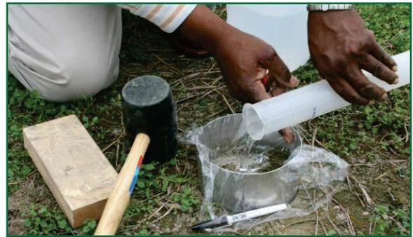
Figure 2.—Water is poured into plastic-lined ring.
