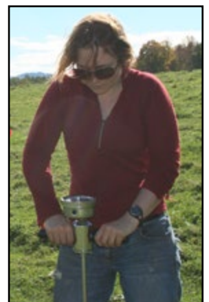
Measuring soil compaction using penetrometer. (University of Vermont)
